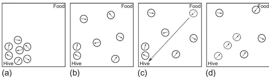
**Figure 13.8** The four stages of Biomimicry Foraging. (a) All robots start at the nest location. (b) The robots randomly disperse through the environment looking for a food location. (c) A robot that has found food returns to the nest location by the shortest possible path. (d) The food location is communicated to other robots and they start to exploit this food source.
