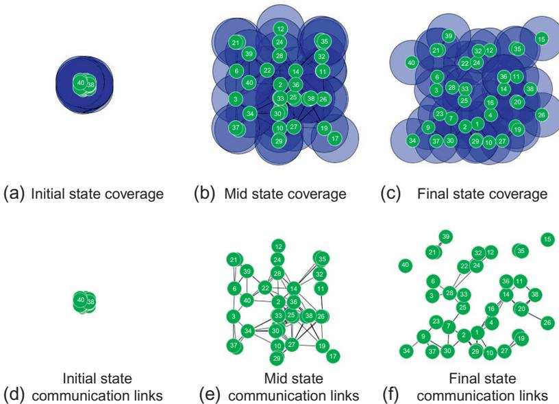
**Figure 13.10** Spread of an MRS of 40 robots: (a)–(c) area coverage and (d)–(f) connectivity of the communication links when network connectivity is assured by *BeePCo*.
