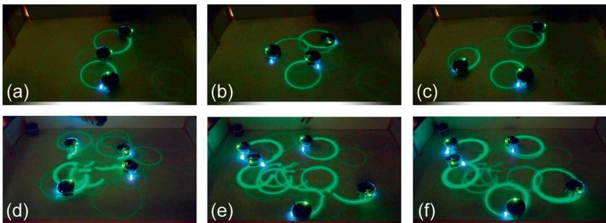
**Figure 13.6** Vision-based stigmergic coverage using glowing trails. (a)–(c) Three robots converging into a stable configuration and forming three singular territories. (d)–(f) Five robots converging into a stable configuration and forming five singular territories.
