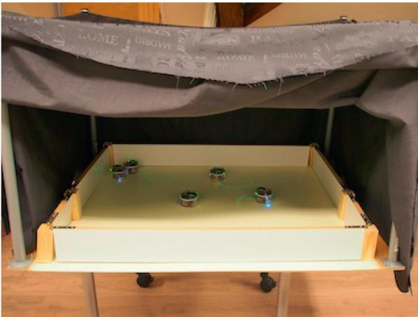
**Figure 13.5** Darkroom with glow-in-the-dark floor, where the e-puck robots circle around and emit UV light onto the floor.
