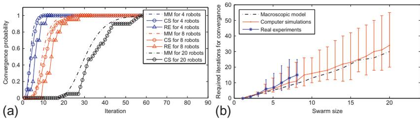
**Figure 13.7** Model verification (a) convergence probability in different iterations (MM: Macroscopic Model, CS: Computer Simulations, RE: Real Experiments). (b) Effects of swarm size on convergence time.
