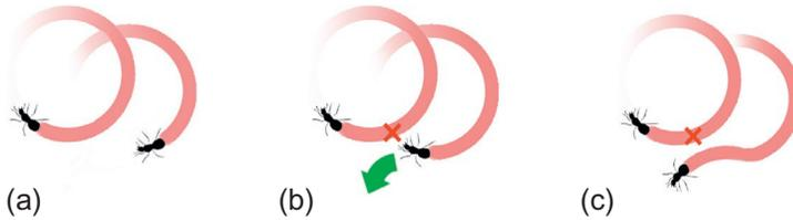
**Figure 13.2** StiCo coordination principle: (a) Robots circle around. (b) The right robot detects pheromone. (c) The right robot changes circling direction.
