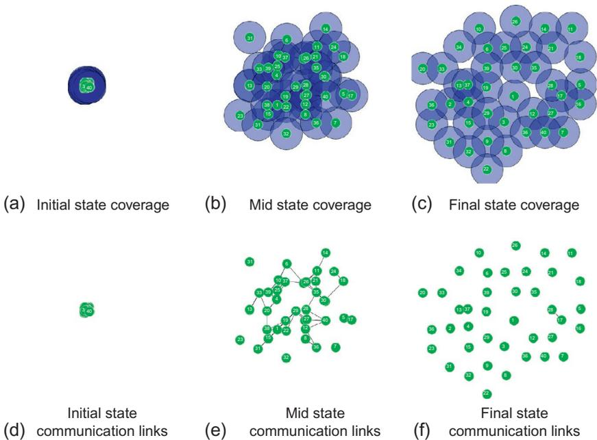
**Figure 13.11** Spread of an MRS of 40 robots: (a)–(c) area coverage and (d)–(f) connectivity of the communication links when network connectivity is assured by *BeePCo*.
