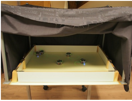
Figure 6: Darkroom with glow-in-the-dark floor, where the e-puck robots circle around and emit UV light onto the floor.
